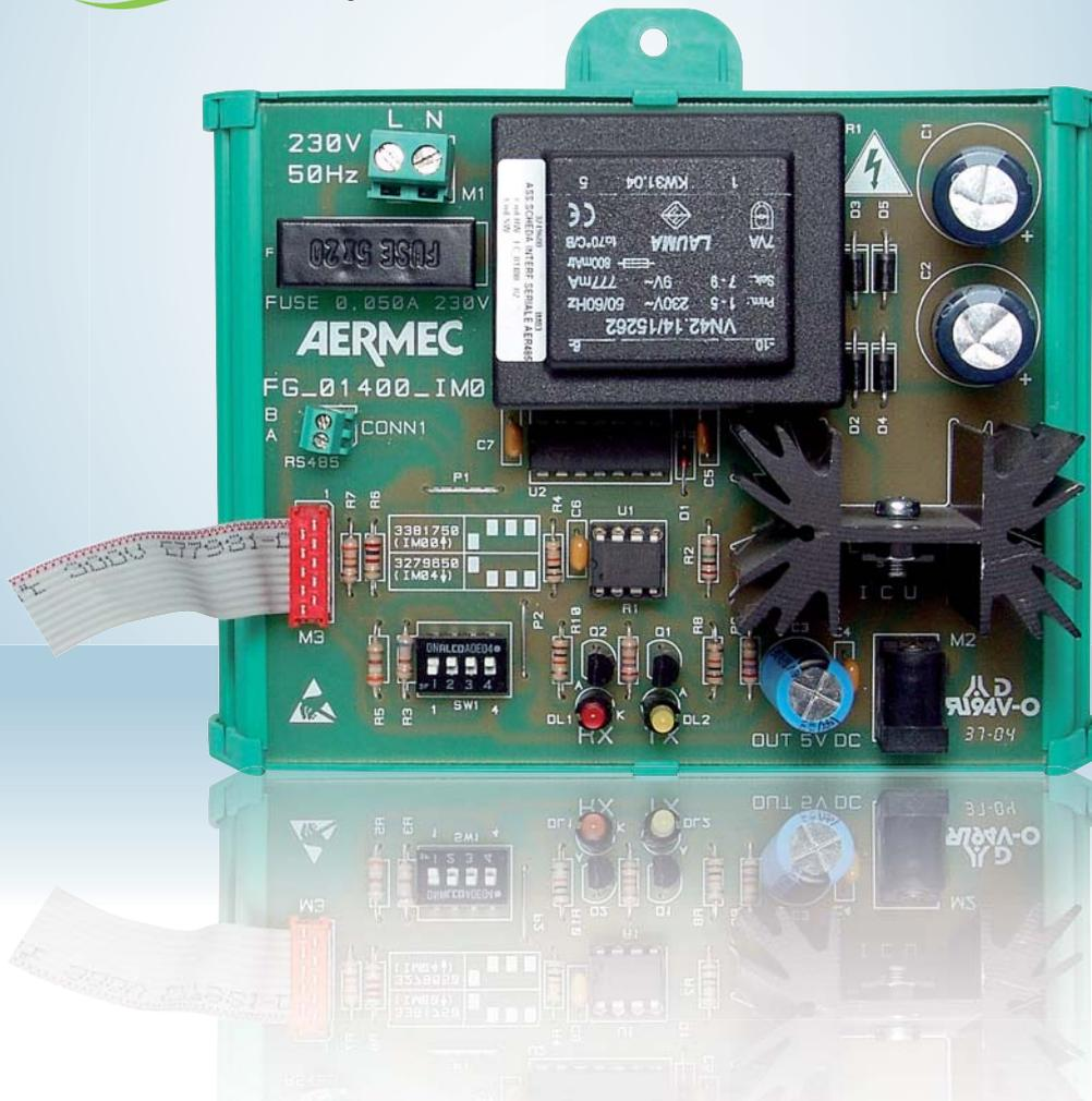
Interfaccia seriale per schede chiller • Serial interface for chiller cards
